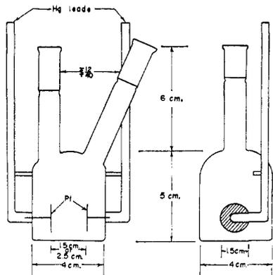
Figure 7. Conductivity cell for kinetic experiments.
