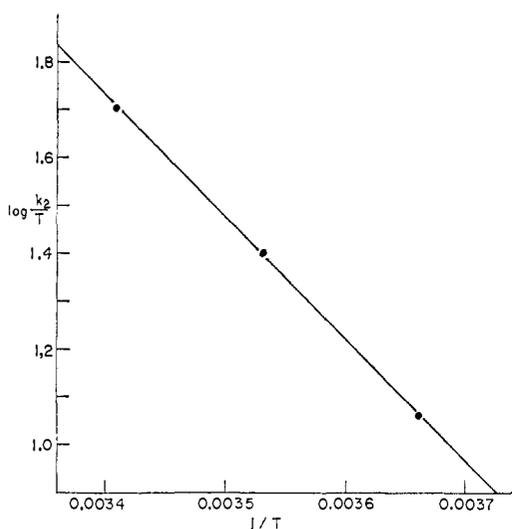
Figure 3. Enthalpy of activation plot ( $\log k_2/T$  vs.  $1/T$ ) for neutralization of 1-*p*-nitrophenyl-1-nitroethane (excess) at 0, 10, and  $20^\circ$ , respectively.
