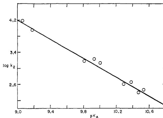
**Figure 5.** Brønsted correlation of the neutralization constants ( $\log k_2$ , 20°) and the ionization constants ( $pK_a$ , 20°) of substituted 1-phenyl-1-nitroethanes; series B,  $\beta = 1.167$ , standard correlation coefficient 0.991, standard deviation 0.054, >99.90% probability  $\beta > 1.0$ .
