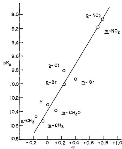
Figure 1. Hammett correlation of the ionization constants ( $pK_A$ ) of *meta*- and *para*-substituted 1-phenyl-1-nitroethanes at 20° in 50% (vol) dioxane-water with  $\sigma$  constants;  $\rho = 1.62$ ; correlation coefficient 0.977.
